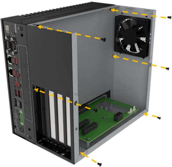
Figure 3-16: Secure TXC-XM81-4S to the Chassis
