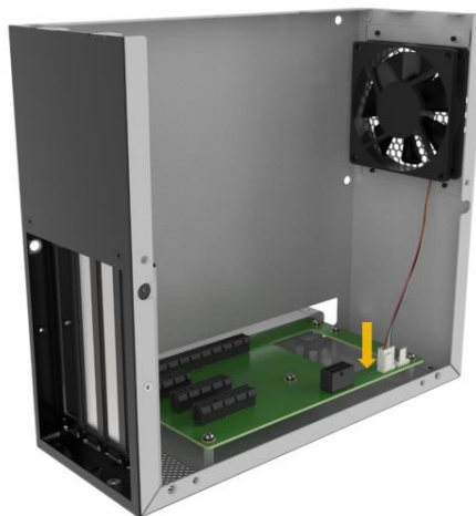
Figure 3-30: Install Fan Cable
