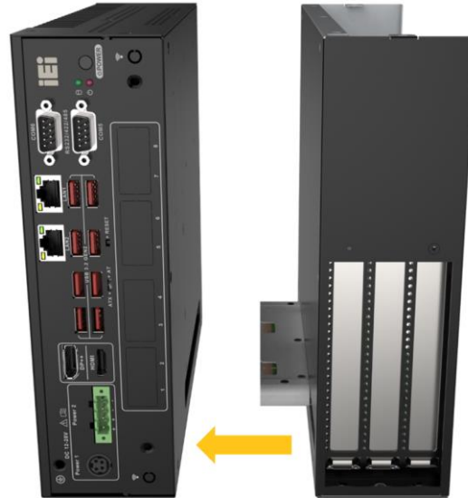
Figure 3-7: Install TXC-XM81-3S to the Host
