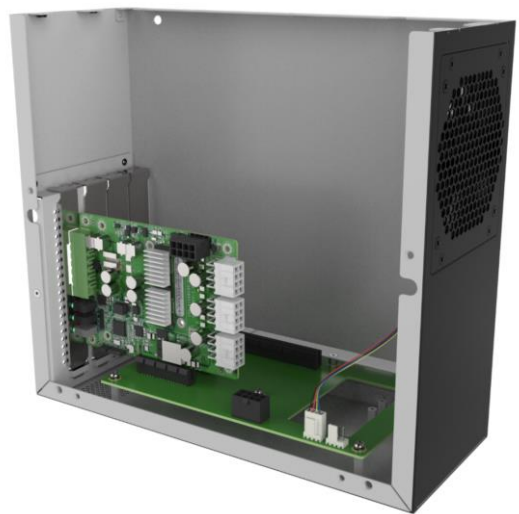
Figure 3-39: Install power module
