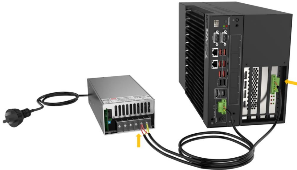
Figure 3-42: Connect with Power Supply
