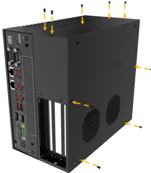
Figure 3-9: Install Cover Screws of TXC-XM81-3S
