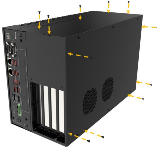
Figure 3-25: Install Cover Screws of TXC-XM81-G1
