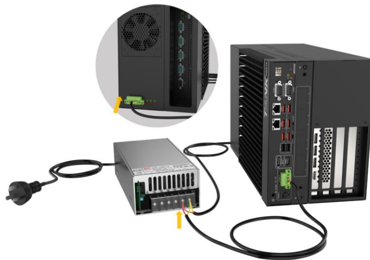
Figure 3-37: Connect with Power Supply
