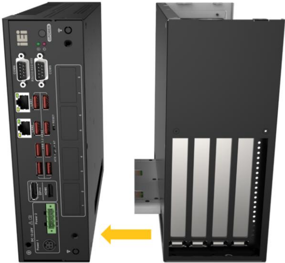
Figure 3-15: Install TXC-XM81-4S to the Host
