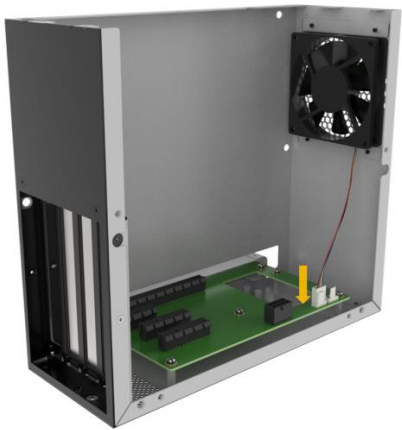
Figure 3-6: Install Fan Cable
