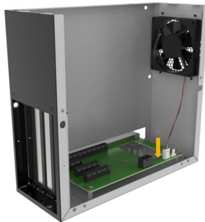
Figure 3-14: Install Fan Cable
