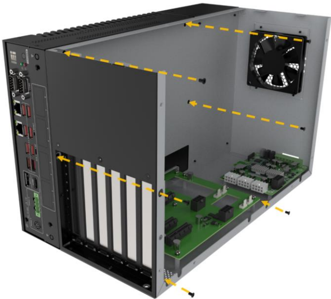
Figure 3-32: Secure TXC-XM81-G2 to the Chassis
