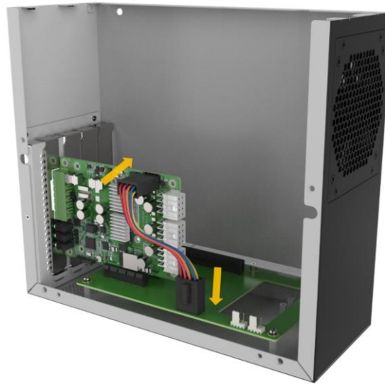
Figure 3-40: Connect Power Cable to Backplane
