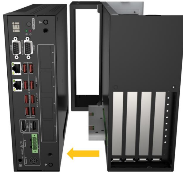
Figure 3-23: Install TXC-XM81-G1 to the Host
