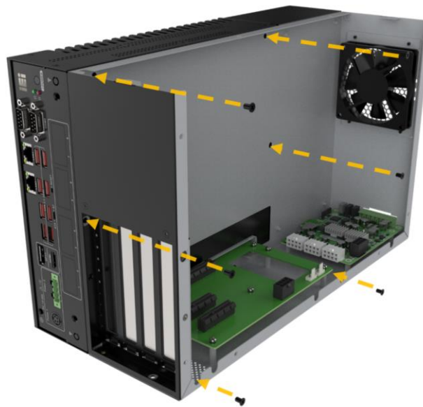
Figure 3-24: Secure TXC-XM81-G1 to the Chassis
