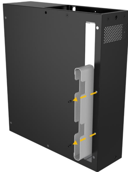
Figure 3-11: Remove the Gold Finger Protection Cover of TXC-XM81-4S
