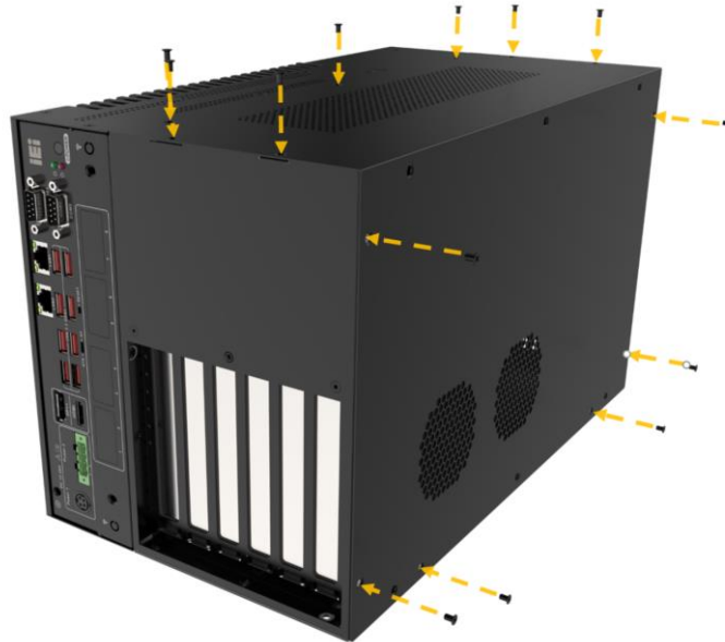
Figure 3-33: Install Cover Screws of TXC-XM81-G2
