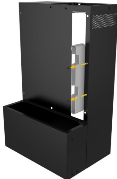
Figure 3-19: Remove the Gold Finger Protection Cover of TXC-XM81-G1
