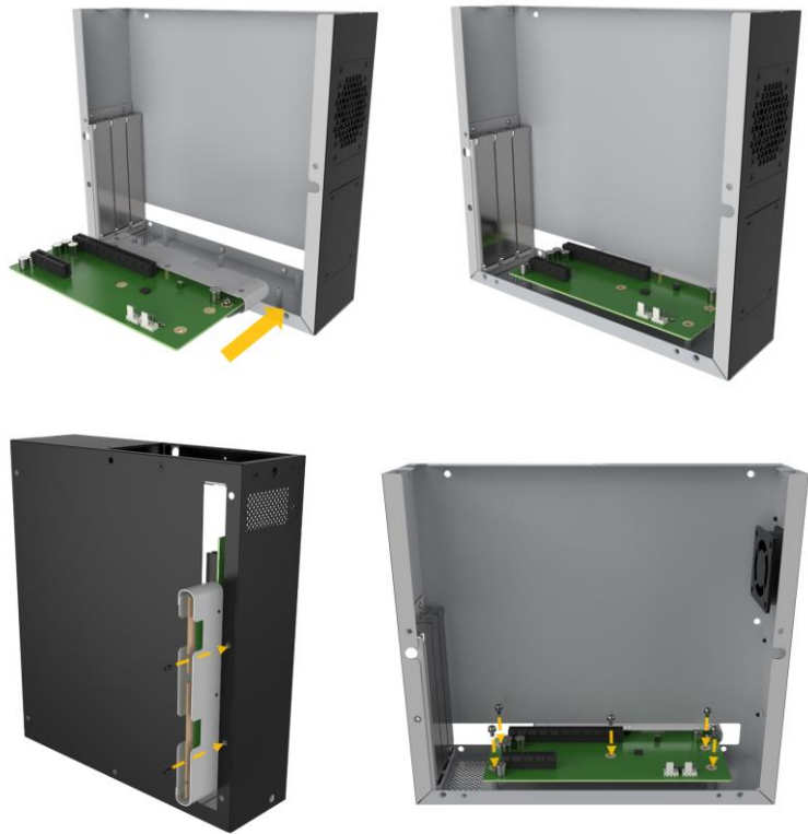
Figure 3-5: Install Backplane into TXC-XM81-3S
