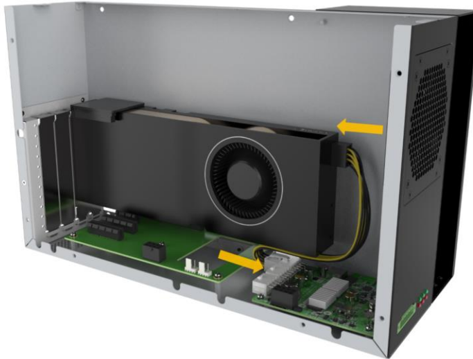
Figure 3-36: Connect Power Cable to Add-on Card
